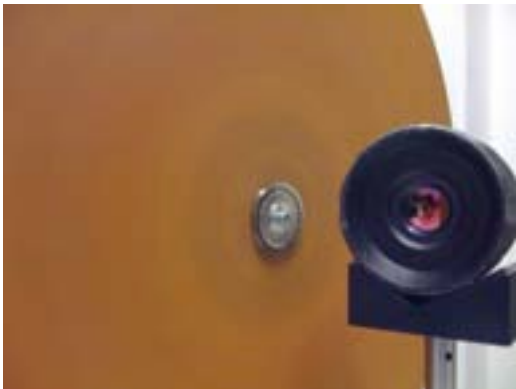
Fig. 1: Corroded steel disc spinning behind the germanium zoom lens of the infrared detector
