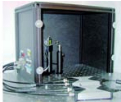
Fig. 2: Measurement box and two compact digital oscilloscopes.
