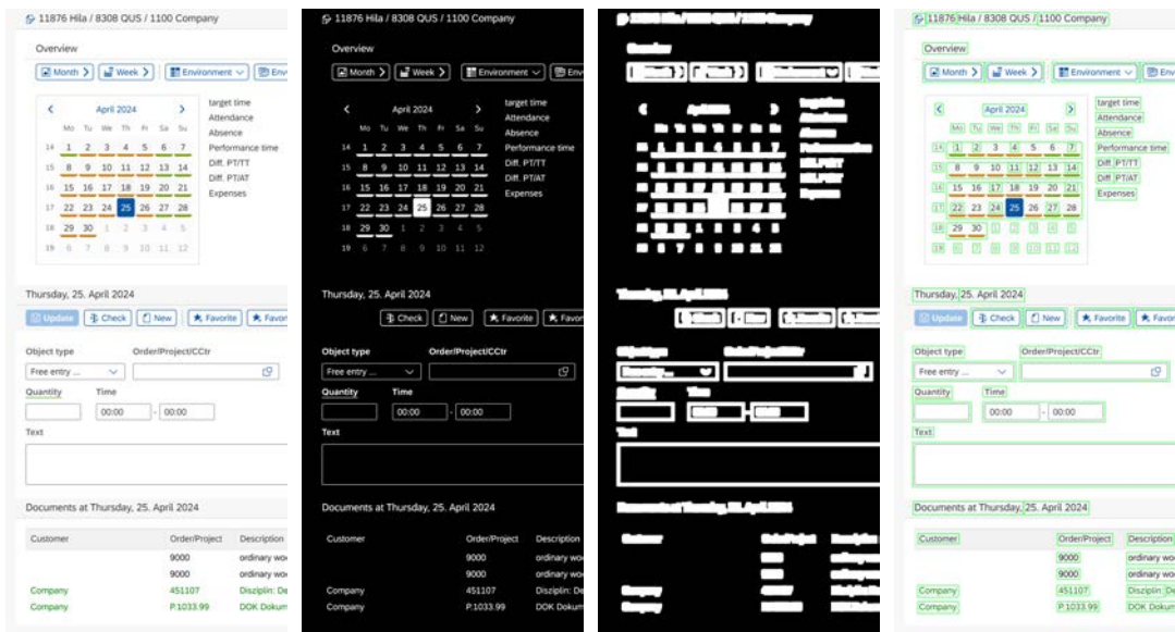
(A) raw image (B) grayscaled image (C) dialated image (D) processed image
