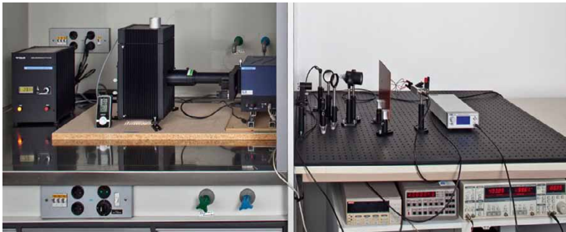
Fig. 1: Experimental setup for spectral photocurrent characterization of solar cells.
